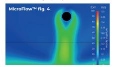
Air permeability 200 m<sup>3</sup>/h/m<sup>2</sup> [10 CFM/ft<sup>2</sup>] at 120 Pa [0.48 inwg], cooling with  $\Delta$ T of -5 K [-9.0°F]. Micro-perforation enables a higher cooling capacity while keeping the occupied zone draft-free.
