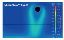
Air permeability 200 m<sup>3</sup>/h/m<sup>2</sup> [10 CFM/ft<sup>2</sup>] at 120 Pa [0.48 inwg], cooling with  $\Delta$ T of -1 K [-1.8°F]. High level of comfort is achieved.
