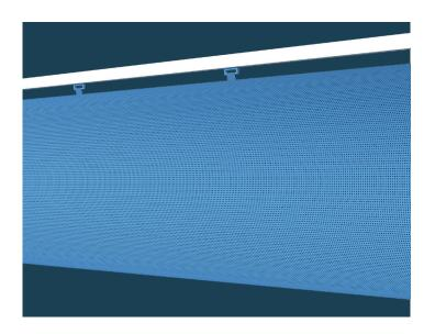
Examples of CFD simulations with MicroFlow<sup>™</sup> at 3 m [≈10 ft] above floor level. The occupied zone is indicated by the black line 1,8 m [≈6 ft] above floor level. When the cold air exits the duct, it moves downward due to thermodynamic forces and merges into a uniform airflow that gains momentum as it moves away from the duct.
