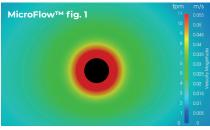
Air discharge through MicroFlow™ of permeability 200 m³/h/m² [10 CFM/ft²] at 120 Pa [0.48 inwg]. Isothermal conditions.
