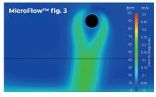
Air permeability 200 m<sup>3</sup>/h/m<sup>2</sup> [10 CFM/ft<sup>2</sup>] at 120 Pa [0.48 inwg], cooling with  $\Delta$ T of -3 K [-5.4°F]. Increased cooling capacity and draft still avoided.
